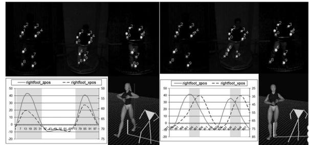
Figure 4. X-axis and Y-axis position of the right foot during forward walking (left) and left rotation gait (right)
